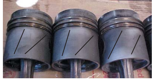
Fig. 1.3.1 Inclined marks at the piston skirt region
