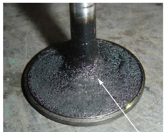
Fig. 11.9.2 Inlet valve contaminated by lubricating oil due to excessive clearance between valve and valve guide or malfunction of oil seal
