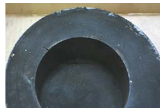
Fig. 2.13.6 Cracks at combustion bowl rim
