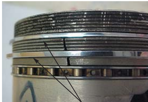
Fig. 2.15.2 Fractured lands in piston (Otto-cycle engine)
