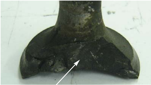
Fig. 11.6.1 Breakage of part of the head
