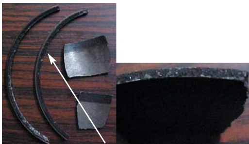
Figs. 5.1.2 and 5.1.3 Dry cylinder liner. Carbonized flange region
