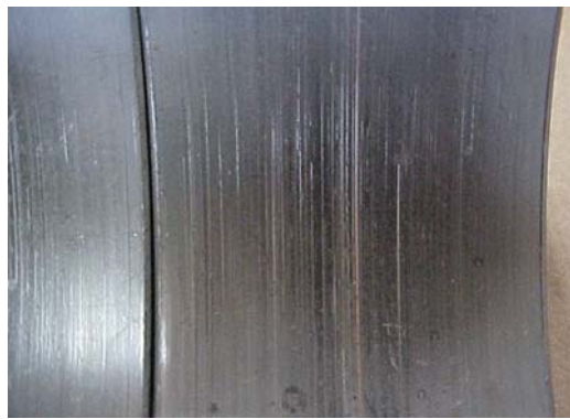
Fig. 8.2.6 Contaminated con rod bearing with circumferential scratches
