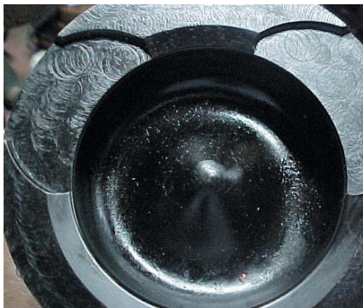
Fig. 2.13.2 Machining marks on piston crown and valve recesses
