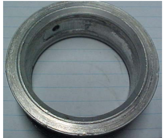
Fig. 8.1.2 Totally worn-out flange
