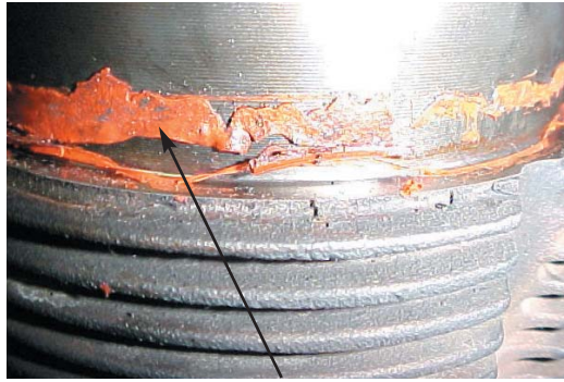
Fig. 4.1.2 Silicone at the lower base of the cylinder liner
