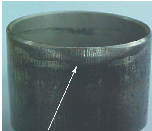
Fig. 10.3.2 Inclined bushing mounting mark
