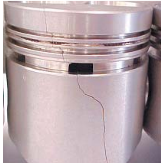
Fig. 2.14.3 Part which has been cracked during con rod fitting
