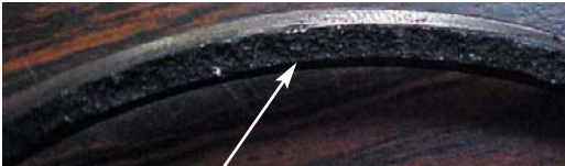
Fig. 5.1.4 Flange region of a carbonized cylinder liner
