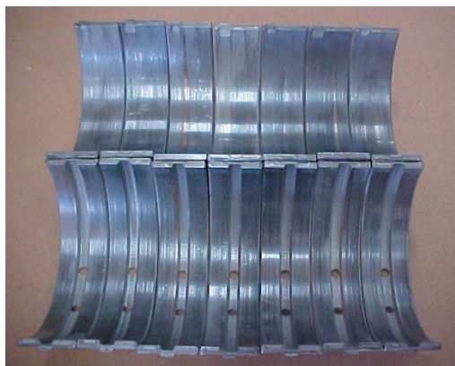
Fig. 8.2.4 Contaminated main bearings with circumferential scratches
