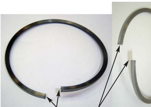
Fig. 3.4 Displaced butts due to incorrect mounting
