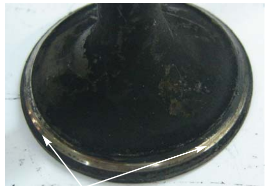
Fig. 11.9.1 Irregular seating area
