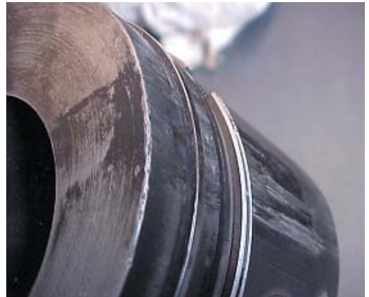
Fig. 2.6.6 Irregular spraying done by the nozzle
