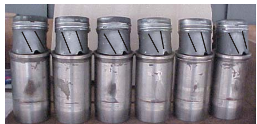
Fig. 1.3.4 Inclined marks at the piston skirt region
