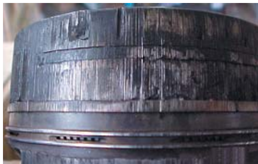
Fig. 2.7.8 Scuffing started at the top land
