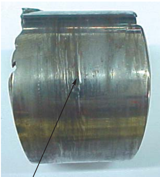
Fig. 10.3.1 Incorrect bushing mounting mark
