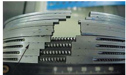
Fig. 3.5.7 Considerable wear on the third groove
