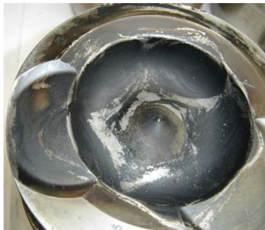
Fig. 2.6.3 Irregular spraying done by the nozzle
