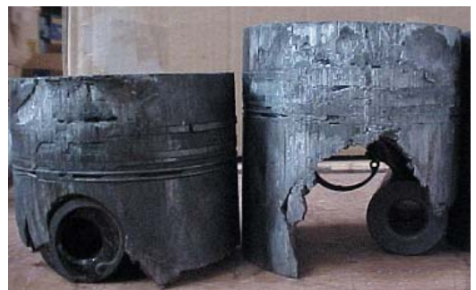
Fig. 2.6.7 Scuffing started at the top land, followed by rupture at the pin boss
