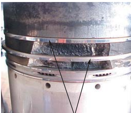
Fig. 2.15.4 Fractured lands in piston (Diesel-cycle engine)
