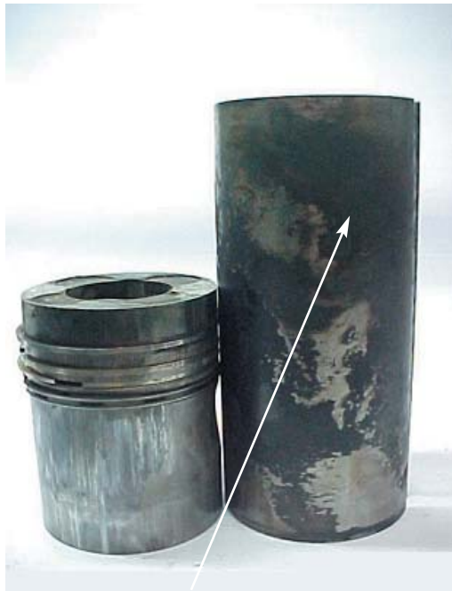
Fig. 5.2.1 Dark marks on internal side of cylinder liner, identifying the lack of interference with the housing
