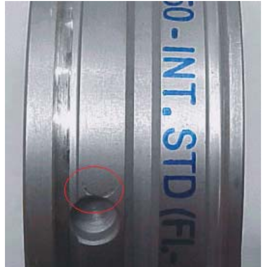
Fig. 8.13.1 Pin mark on external bearing side
