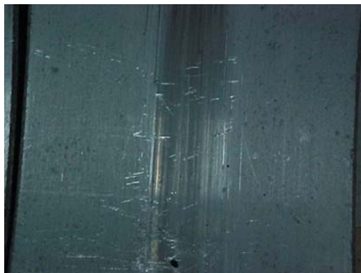
Fig. 8.2.8 Contaminated con rod bearing and circumferential scratches in the lubricating hole direction
