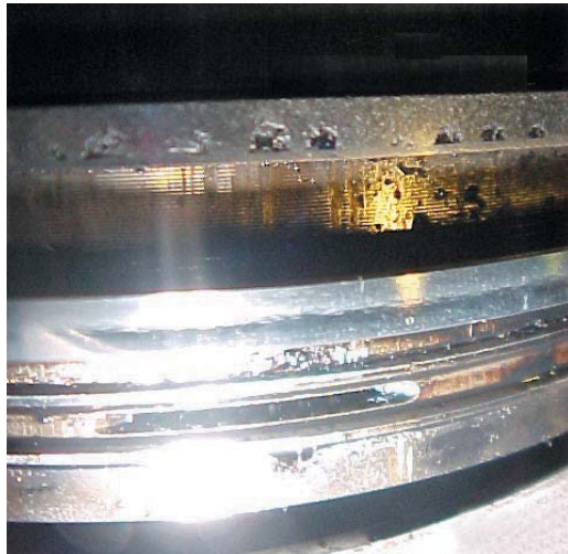
Fig. 3.6.5 Flaking-off of the piston ring coating
