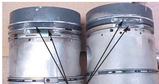
Fig. 2.15.3 Fractured lands in piston (Diesel-cycle engine)
