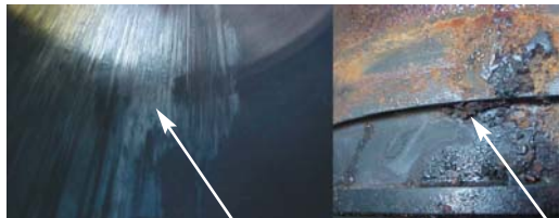
Figs. 5.2.2 and 5.2.3 Scuffing originated by O'ring displacement. Impurities in the cylinder liner O'ring housing
