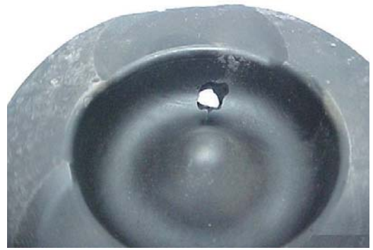
Fig. 2.7.10 Destruction of the crown and the pin boss region, due to irregular injection
