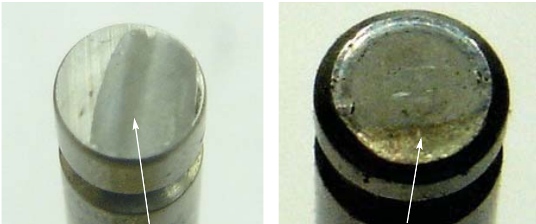
Fig. 11.9.4 Marks indicating that the valve hasn't rotated. Rocker arm deficiency
