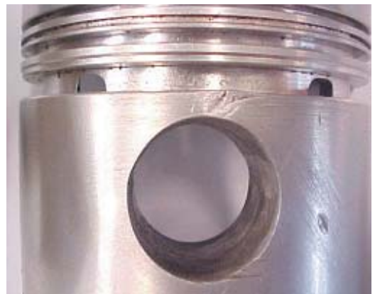
Fig. 2.14.4 Irregular mark, close to the pin boss
