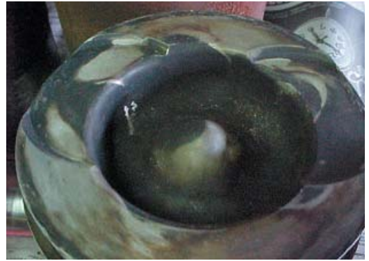
Fig. 2.6.4 Irregular spraying done by the nozzle
