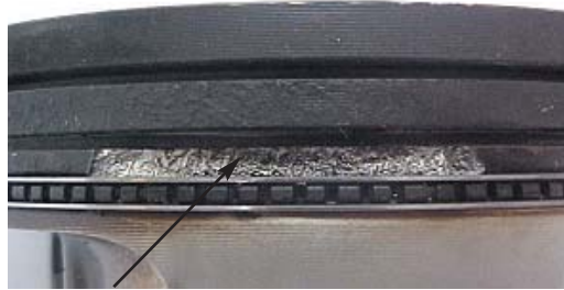
Fig. 2.15.1 Broken land in piston (Otto-cycle engine)
