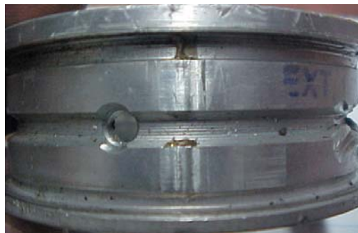
Fig. 8.13 Glue/adhesive on bearing's external lubrication channel
