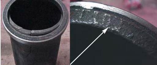
Figs. 5.1 and 5.1.1 Wet cylinder liner. Fractured and carbonized flange region
