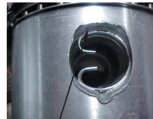
Fig. 1.1.3 Damages caused by circlip
