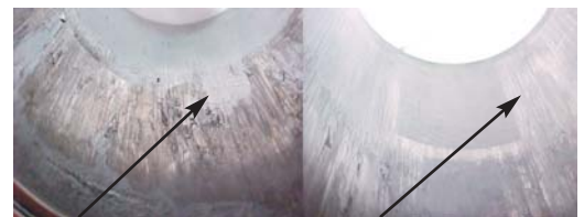
Figs. 5.3.1 and 5.3.2 Scuffing originated by dilution of lubricating oil existent on inner cylinder wall
