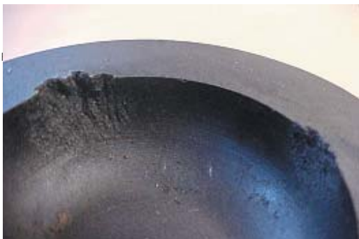
Fig. 2.7.1 Partial destruction of the combustion chamber
