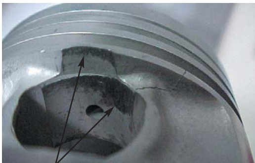
Fig. 2.14.2 Irregular piston pin marks on the bosses during con rod fitting
