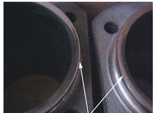
Fig. 4.1.5 Irregular cylinder liner seat on the cylinder head
