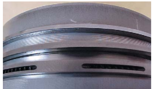
Fig. 3.5.6 Worn-out piston ring of the third groove
