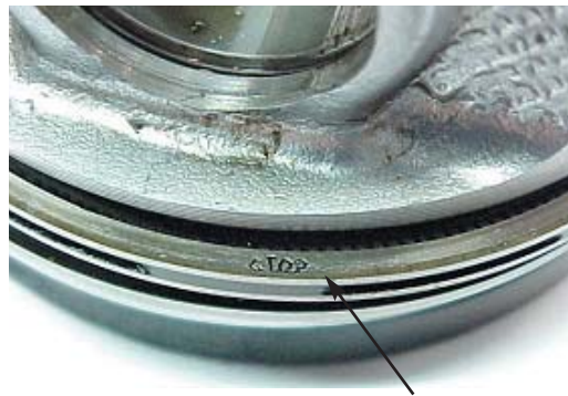
Fig. 3.1 Piston ring mark mounted towards the lower side
