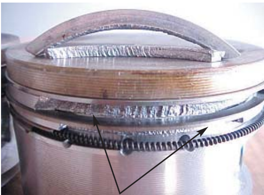
Fig. 2.15 Broken lands in piston (Otto-cycle engine)
