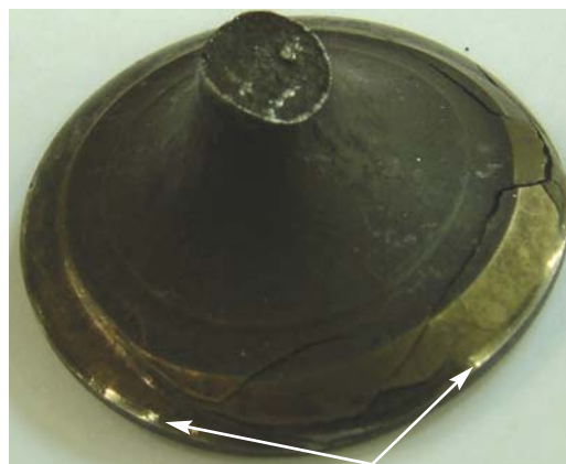
Fig. 11.3.2 Broken valve head at the radius and stem region
