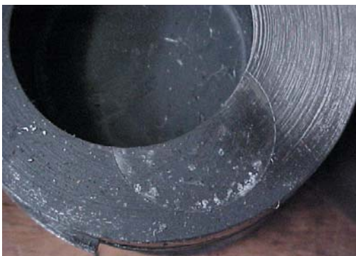
Fig. 2.8.1 Valve mark on machined piston crown
