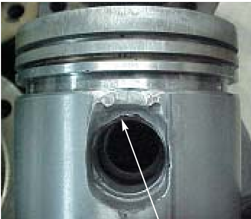
Fig. 6.2 Piston wear, at the bosses and crown region, caused by the circlip
