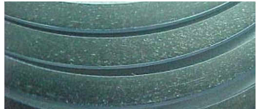
Fig. 3.5.5 Piston ring with abrasive particles on lateral face
