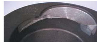
Fig. 2.13.5 Machined valve recess
