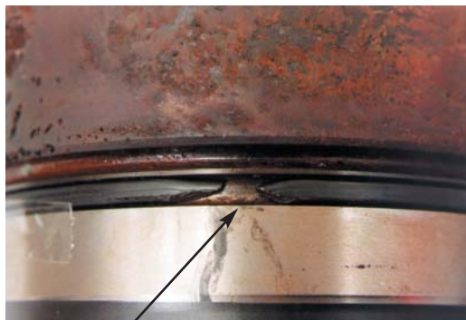
Fig. 5.2.4 O'ring has been cut during cylinder liner fitting in engine block
