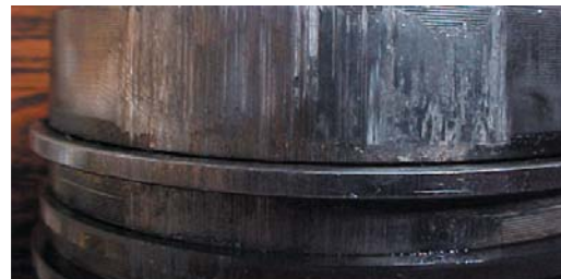
Fig. 2.7.4 Scuffing started at the top land
