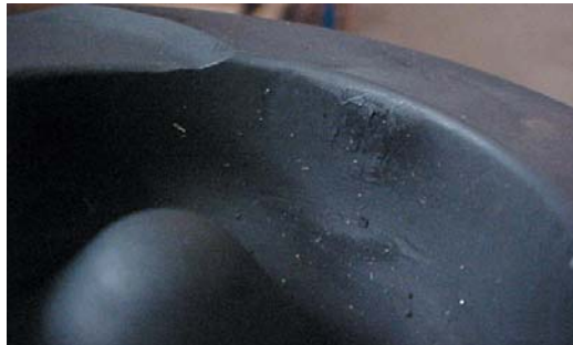
Fig. 2.6.1 Spraying occurs partially out of the combustion chamber
