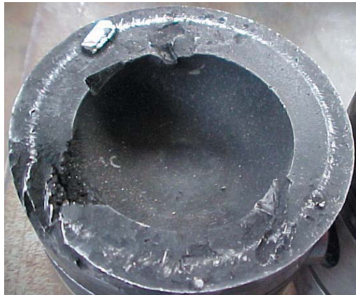
Fig. 2.7.7 Partial destruction of the crown, due to injection defect
