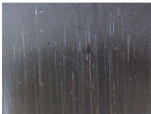
Fig. 8.2.7 Enlarged photo of scratches and odd materials on a bearing
