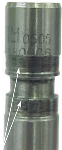
Fig. 11.4.4 Wear at the keeper groove channel caused by irregular keeper
