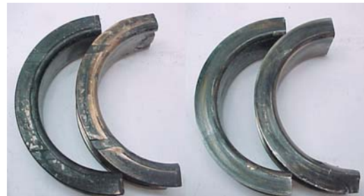
Fig. 8.1.3 Bearing flange front side without wear and back side with wear
