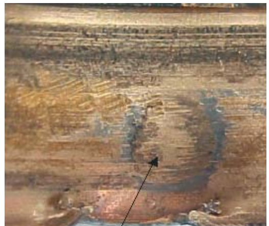
Fig. 10.2.5 Internal mark formed by odd material
