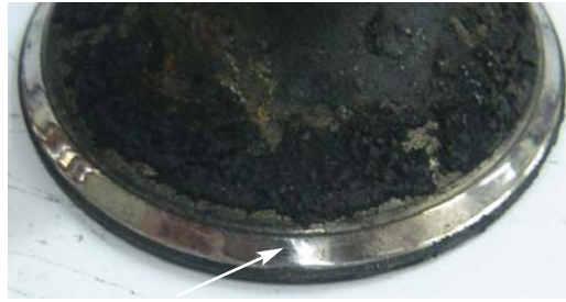
Fig. 11.7.1 Wear at the valve head region
