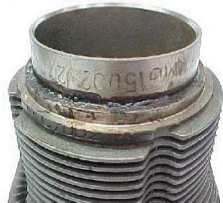
Fig. 4.1.4 Cylinder head was fitted with glue at its lower base
