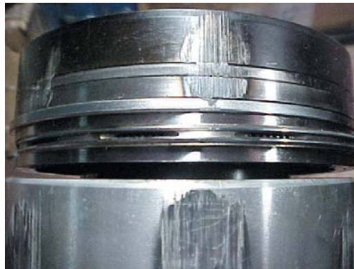
Fig. 2.7.3 Scuffing started at the top land, and extended to the piston skirt
