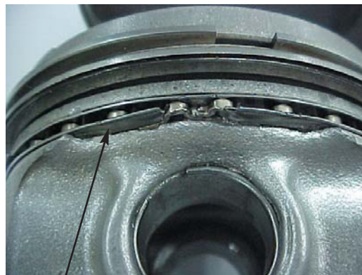
Fig. 1.1.2 Damages caused by circlip
