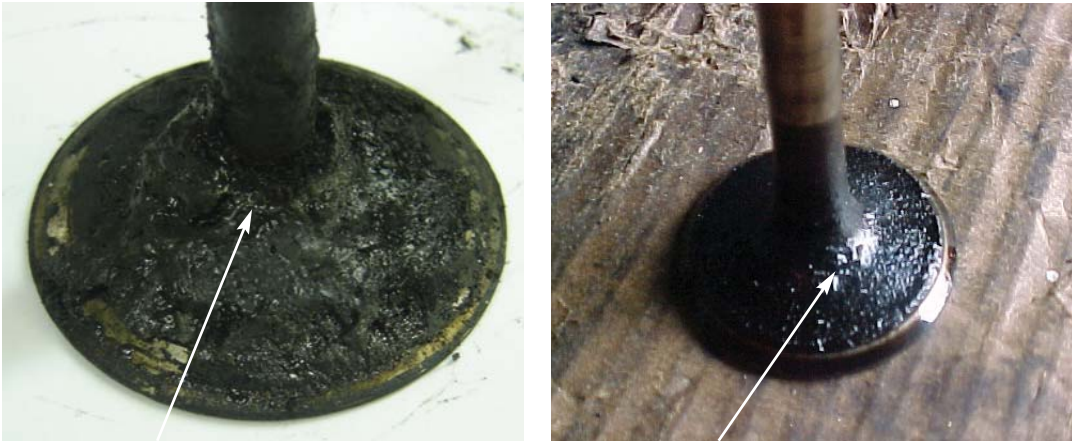
Fig. 11.9.3 Contaminated inlet valve with lubricating oil crust due to excessive clearance between valve and valve guide or malfunction of oil seal
