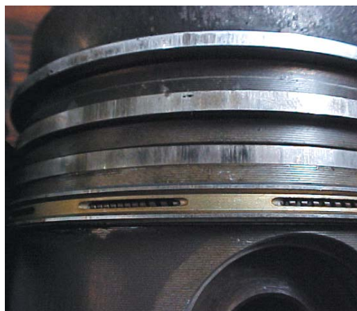
Fig. 2.7.5 Scuffing started at the top land
