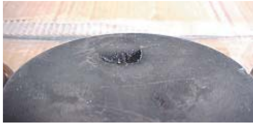
Fig. 2.7.6 Partial destruction of the crown, due to injection defect
