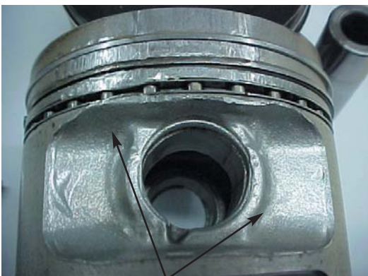
Fig. 1.1.1 Damages caused by circlip
