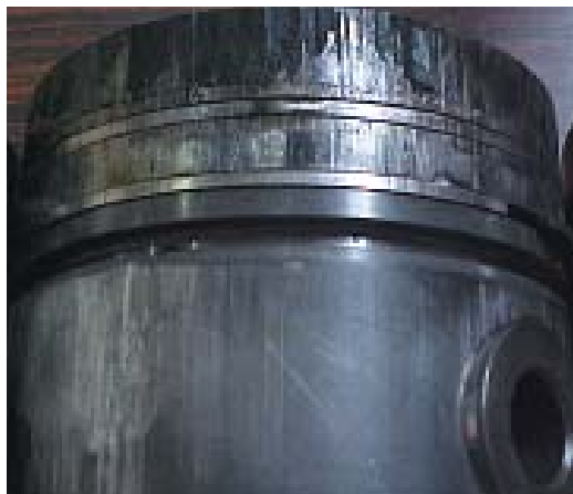
Fig. 2.7.9 Scuffing started at the top land
