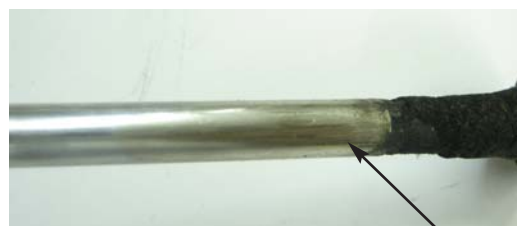
Fig. 11.1.4 Scuffing due to insufficient clearance between valve and valve guide
