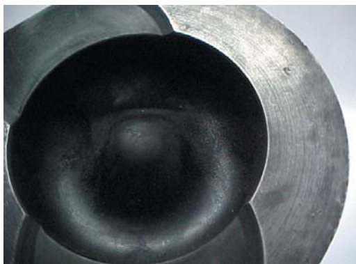
Fig. 2.13.1 Machining marks at piston crown
