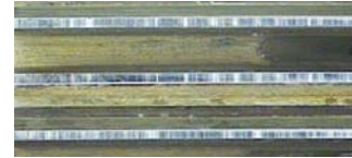
Third groove piston ring. Running face - contact zone with cylinder. 180° from gap
