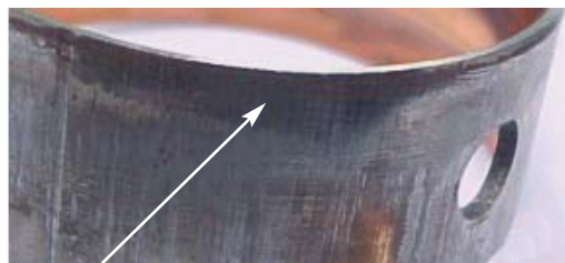
Fig. 10.3.5 Inclined bushing mounting mark
