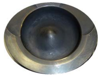
Fig. 2.13.4 Machined valve recess
