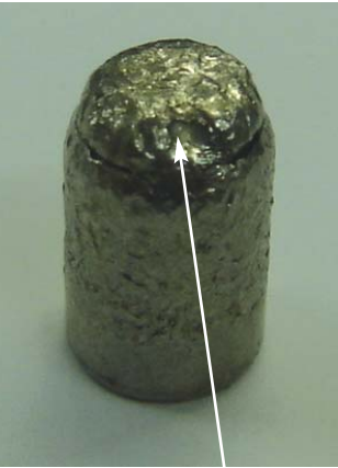
Fig. 11.4.1 Breakage at the keeper groove region
