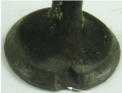
Fig. 11.8.1 Localized disintegration at the seat region
