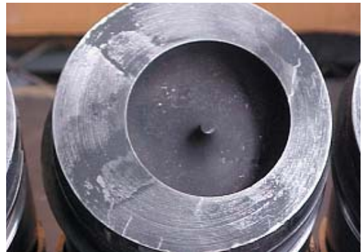
Fig. 2.6.5 Irregular spraying done by the nozzle
