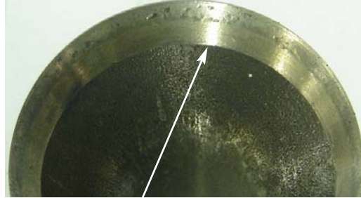
Fig. 11.7.2 Wear at the valve head region
