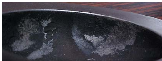
Fig. 2.6.2 Spraying occurs partially out of the combustion chamber
